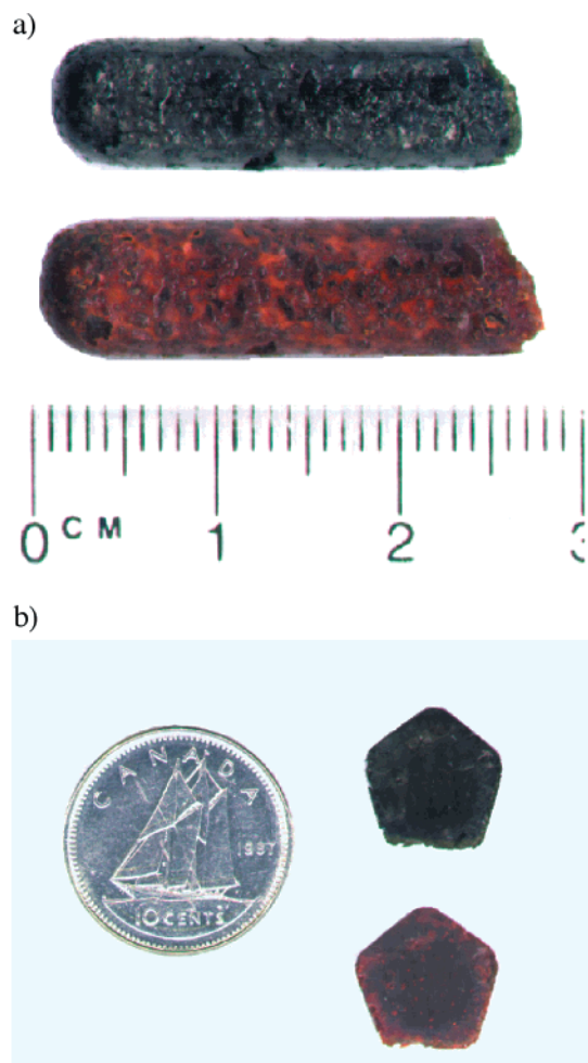
Figure 2. (a) Photograph of a red polymer rod 4 (bottom) and the corresponding pyrolysis product, ceramic 5 (top). (b) Pentagon-shaped polymer 4 (bottom) and the resulting pentagon-shaped ceramic 5 (top).
